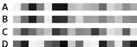
FIGURE 4.6. Illustration of vector similarity, with four sequences of sixteen numbers visualized through color coding. A is 98 percent similar to B, 90 percent similar to C, and unrelated to D. Hypothetically, A and B might result from images of the same dog, C from another dog, and D from, say, a living room.
