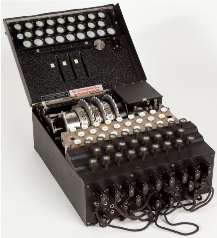
FIGURE 5.1. Notable historical computers. (a) A modern re-creation of the Antikythera mechanism, a special-purpose analog computer used by the ancient Greeks to predict eclipses and other astronomical events. (b) A Hollerith tabulating machine, which helped greatly speed up the 1890 U.S. census and eventually led to the birth of IBM. (c) An Enigma machine used by the Nazis for encrypted communication during World War II.
